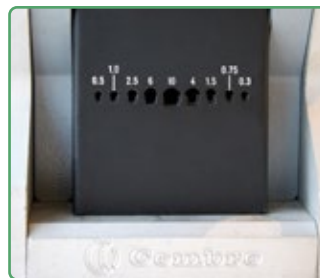
PNB-4KE detail of the crimping zone.
