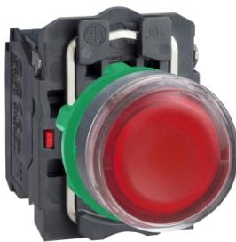
Illuminated push button, Harmony XB5, plastic, flush, red, 22mm, plain lens for BA9s bulb, spring return, lower than 250V, 1NO + 1NC
