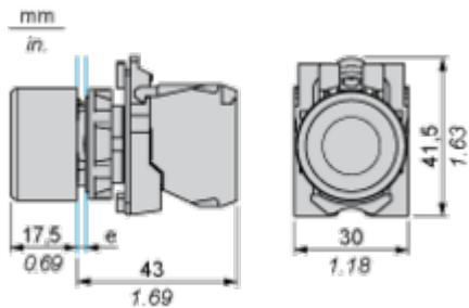
e: clamping thickness: 1 to 6 mm / 0.04 to 0.24 in.
